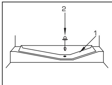
If at any time the defrost water does not drain from the collection channel, check to ensure that no food particles have blocked the drain tube. The drain tube can be cleared by pushing the special plastic plunger provided down the drain tube (2).
