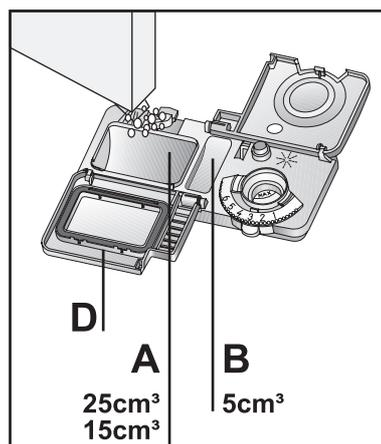
If your dishes are kept unwashed for a long time and the food particles are stuck on the dishes also fill the small container (B) up to 5cm<sup>3</sup>. Depending on the degree of soiling and the water hardness in your area it may be necessary to add more detergent.
